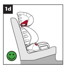
Push the child seat back until it is touching the car's seat back (dia 1d). The cars seat backrest can be moved to a desired angle.
